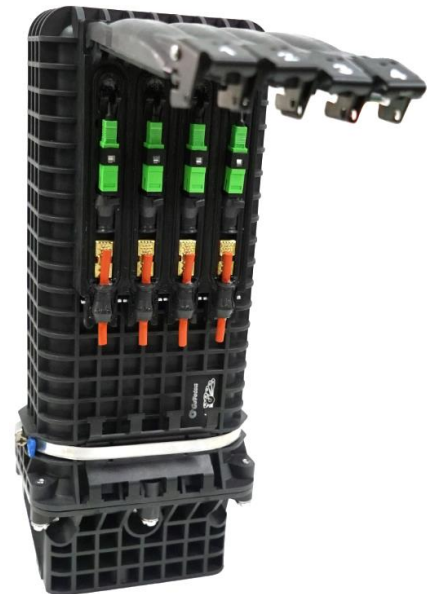
M-CHT (Drop Port Access)
