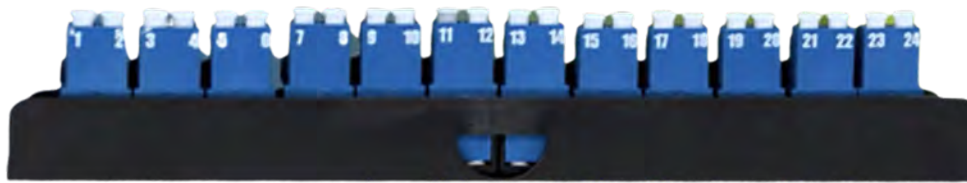
Port Numbering on bottom of duplex LC adapter
