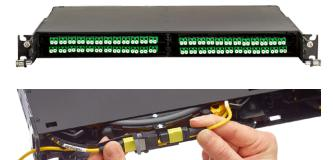
mm cable. The spool capacity not only maximizes the reach distance, but also provides the most flexibility for slack management, virtually eliminating the need for pre-measuring cable lengths. The modular 1RU panel holds up to 96 duplex LC connections. These may be added after first installation, providing ultimate day-two flexibility. The Go!Foton PEACOC 360 is the right-sized quick-deployment connectivity solution for facilities where resources, scalability, and density need to be optimized.
